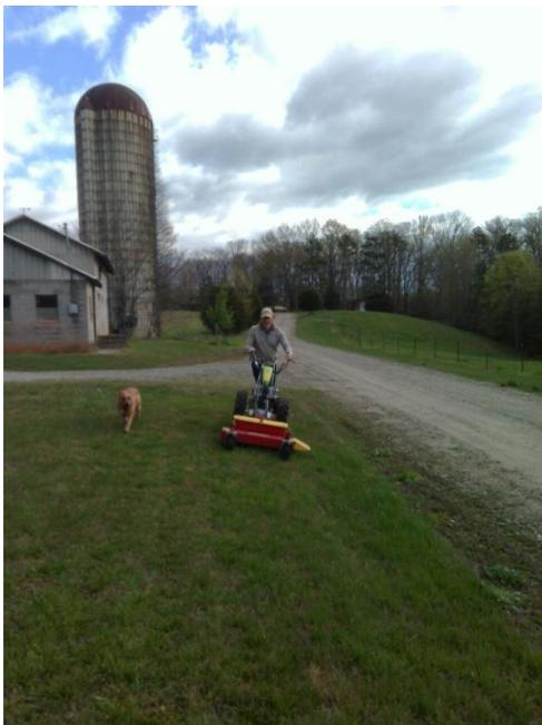
This **33" Zannon** finish mower has dual cutter heads, steering brakes are essential with this machine! This mower definitely requires the steering brakes to aid in maneuvering. **Grillo** makes two larger units than this one, the **G-110** and the **G-131**. The **G-131** is their largest
