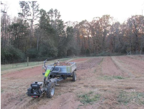
The **Grillo G-107d** with the driven wheel trailer attached making this a 4-wheel drive utility vehicle capable of carrying a 1500# payload, shown here transporting leaves to be tilled into the garden!
