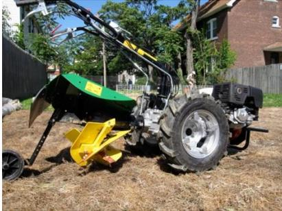
**G-107d w/Berta Rotary Plow** shown attached in “transport mode”, trailing wheel lifts the plow off of the ground.
