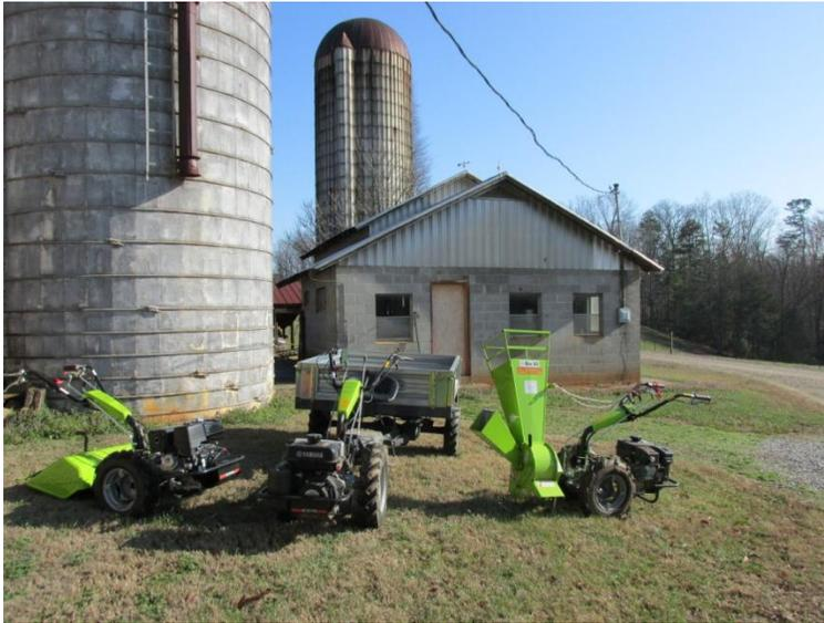
Grillo tractors, left to right, G-107d with 27" tiller attached, G-107d with driven wheel trailer, and G-85d with Carrivaggi chipper/shredder attached.
