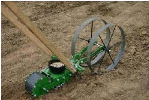
Here the Hoss™ seeder attachment plants corn to the correct depth. Seed depths are adjustable from  $\frac{1}{4}$ " to  $1\frac{1}{2}$ ".
